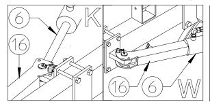
Bring back the latches 16 of the cylinders 6 from working position K to transport position W. To do this, see pages 34-35.
