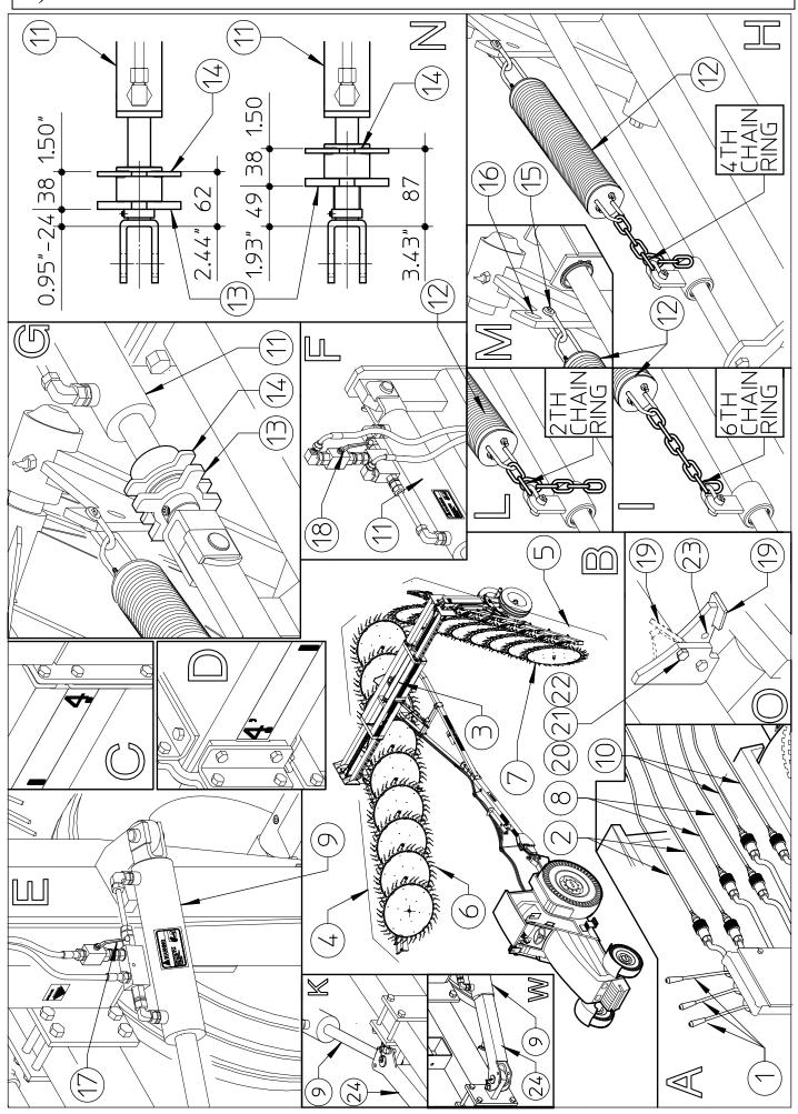
The first thing to do when you are going to work is to open the machine frame. To do this, with the machine running, or at least on a surface that allows the transport wheels to slide sideways, move lever 1 connected to hoses 2 (see box A), which control the cylinders 3 (see box B) that open the sliding crosspieces to a max. width of 4' (see boxes C-D).
